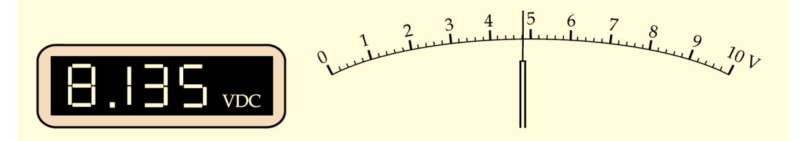
(a) Digital voltmeter display with a 1 mV precision (b) Analog instrument display with a 50 mV precision
